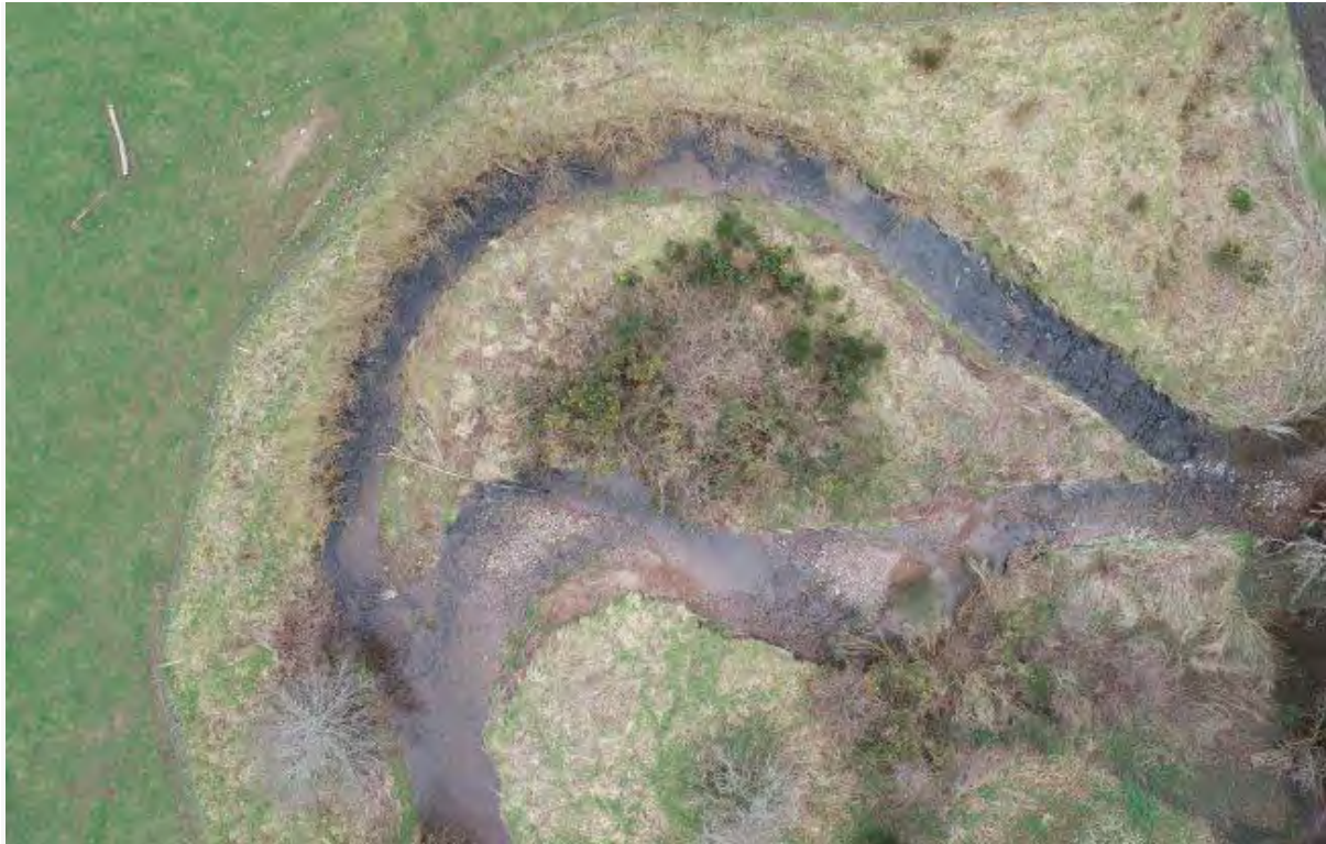
An aerial view of the stabilised bank and the new braided channel that opened up in winter floods 2021/2022. High value land loss has stopped and with it, suspended sediments have reduced
