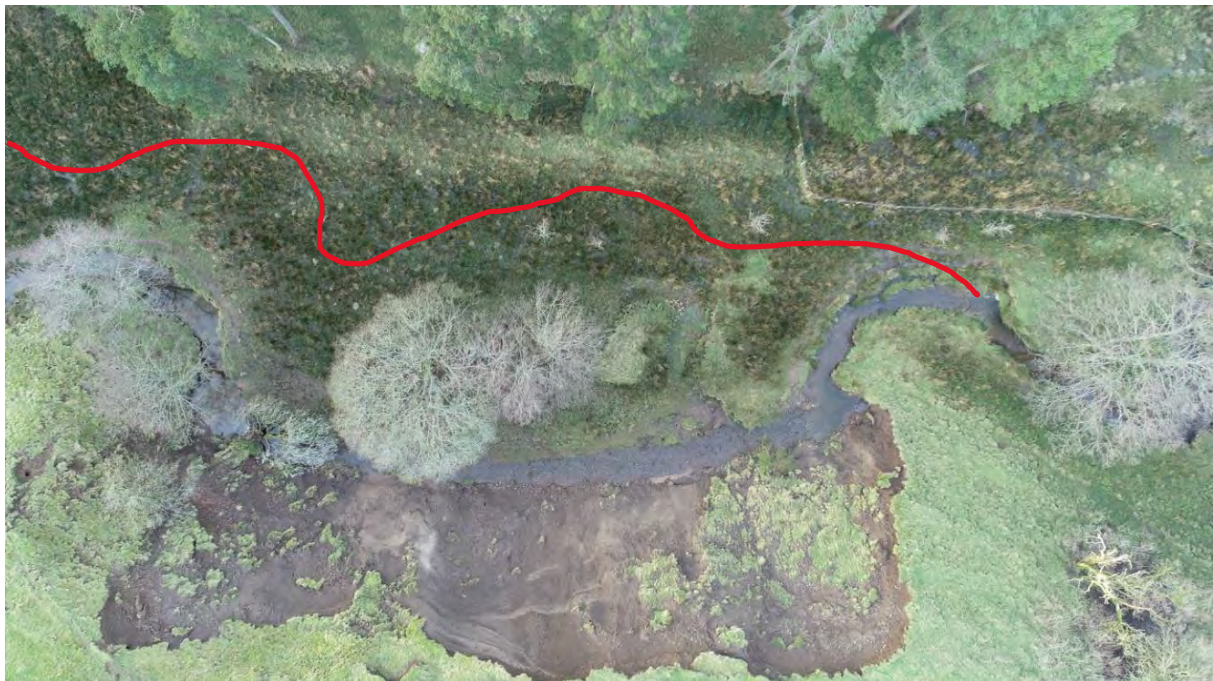
Figure 2: The landslide at Netherton Burn. The proposal includes realigning the burn across the valley floor (approx. location in red), re-joining the natural course downstream of the erosion. Livestock will be excluded from the entire area through new fencing supported by the DSFB.
